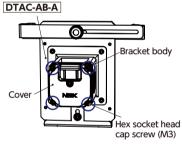
1 Use the hexagon key to loosen 2 Fit the bracket the hex socket head cap screws x 4 at the four corners of the **DTAC-AB-A** cover, and then remove the cover.
