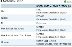
\*1: Due to manufacturing process requirements, couplings may have bores and keyways with or without surface treatment. This does not affect the performance of the couplings.
