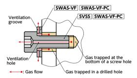
• The ventilation hole easily releases gas trapped in the screw holes of equipment and machines, and supports vacuum drawing of vacuum devices.
